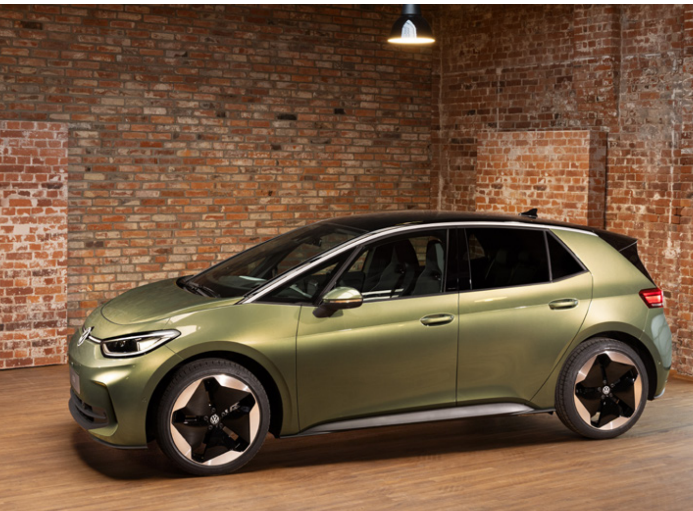
Steeply sloping A-pillars, the flowing roof line and the drawn-in C-pillars give the ID.3 an excellent drag coefficient.
