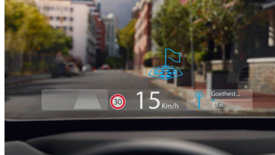
Information on the AR head-up display appears to be ten metres ahead of the vehicle.
